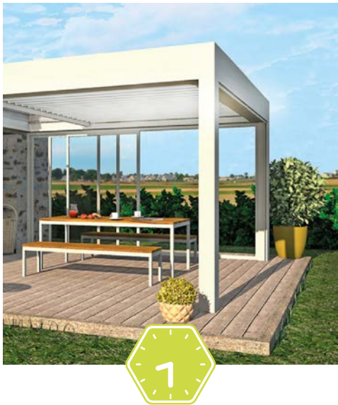
The sun rises. The blades of the pergola open at 90° in order to let the light in.
